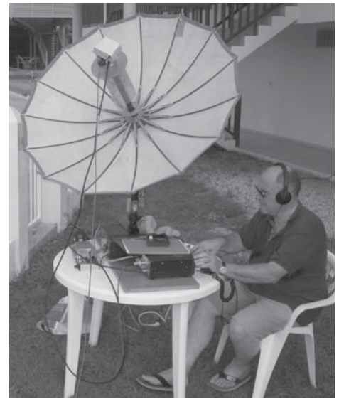
Jean, F6CBC, operating AO-40 Mode L/S from French Guiana using a 1.2 meter Inmarsat umbrella dish
